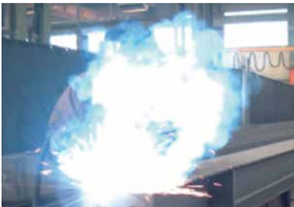
Previously: Severe smoke development with conventional arc.
