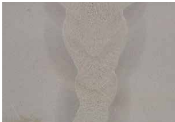
FOCUS.PULS - More layer welding with reduced opening angle (25°). Highest welding seams safety (see polished cut image). The result counts.
