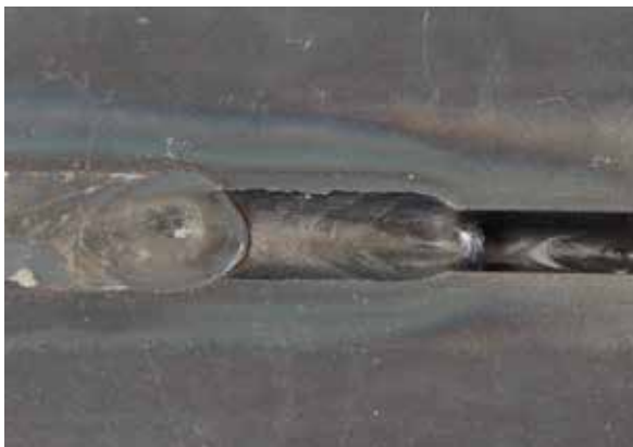
FOCUS.PULS - More layer welding with reduced opening angle (25°). Highest welding seams safety (see polished cut image). The result counts.
